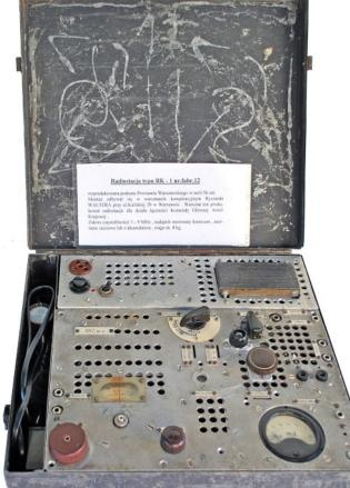
The RK 1 on the photo above was a partial rebuild using an original metal box and almost bare donor set, fortunately still with most of the engraved inscription plates. The AC mains power supply unit at the top was a reconstruction. The meter in the right hand bottom was not original, replacing an original rather large Aerial Coupling knob.
